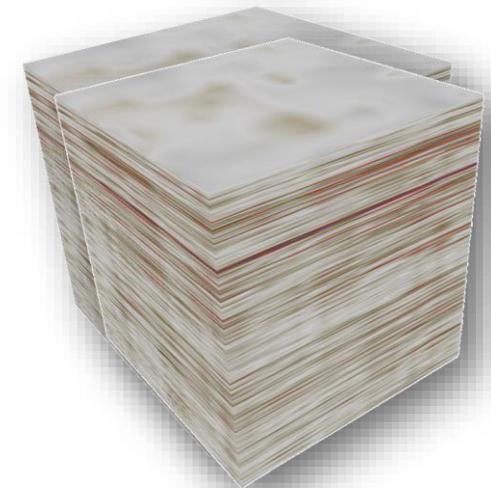
4D seismic time lapsed volumes
